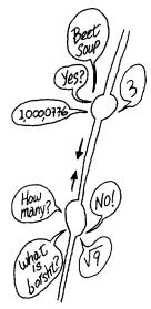
A given, pair of nodes may exchange Several independent Messages for simultaneous users with different interests
